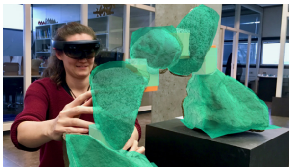
Fig. 7: Irregular shape assembly in AR. This figure was produced by B.Wibranek and O.Tessmann in Technique University Darmstadt, DDU(Digital Design Unit) in 2019 [27], and it summarized the AR setup allowed users to switch parts on and off depending on the stage of assembly. The permission to re-use the figure has been granted by the author and the publisher.
