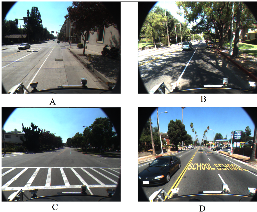
Figure 1. Example cases where extracting lane markings is challenging (A) patched road; (B) Shadow; (C) cross walk; (D) road markings (adopted from [18]).
