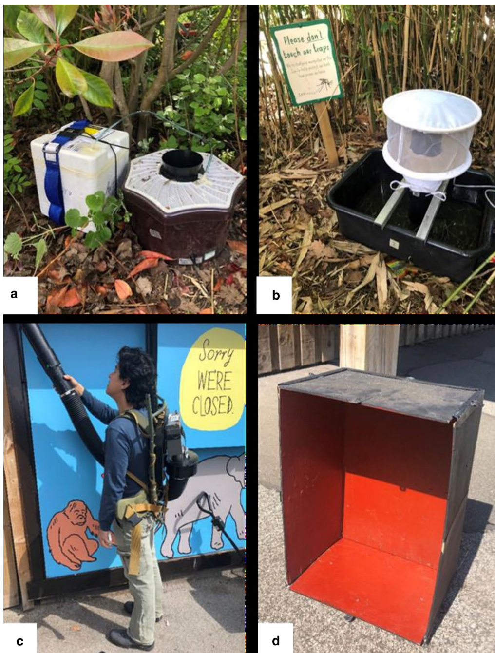
Fig. 1 Trapping methods used for mosquito sampling. a BG-Mosquitaire trap (upgraded with dry ice for the 2019 season); b CDC-Gravid trap model 1712; c Improved CDC-Backpack Aspirator model 1412 (only used in 2019); d resting box trap (only used in 2019). Pictures by FT
