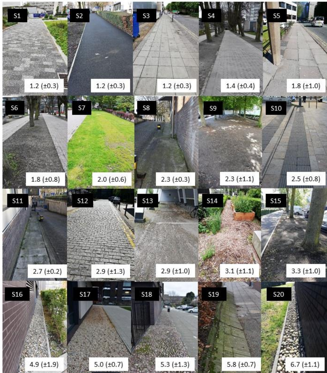
Figure 1: Images showing the 20 surfaces (S1 – S20) used for this study. Surfaces are ordered by the average rating of surface complexity produced from the perceptual rating study from S1 = least complex to S20 = most complex. Surfaces were rated using a scale from 1 (smooth / stable) to 10 (rough / unstable). Average ( \pm SD) perceptual ratings are shown for each surface. Further details about the surfaces are given in the supplementary material (5.7.1).
