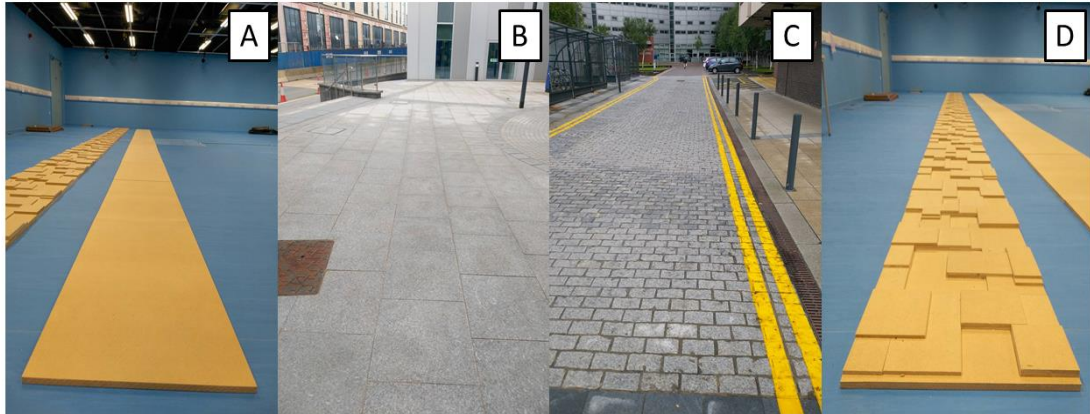
Figure 1: Images showing the four surfaces: (A) indoor, flat, (B) outdoor, paved (C) outdoor, cobbled and (D) indoor, uneven. To estimate surface roughness, we used a clinometer to take 20 measurements of the height change between a pair of points that were 15cm apart. This was done at 30cm intervals along each surface. The mean ( \pm SD) height change was 1.8^\circ (\pm 0.5^\circ) for the indoor, flat surface, 1.9^\circ (\pm 0.5^\circ) for the outdoor, paved surface, 2.5^\circ (\pm 1.9^\circ) for the outdoor, cobbled surface and 7.5^\circ (\pm 2.6^\circ) for the indoor, uneven surface.
