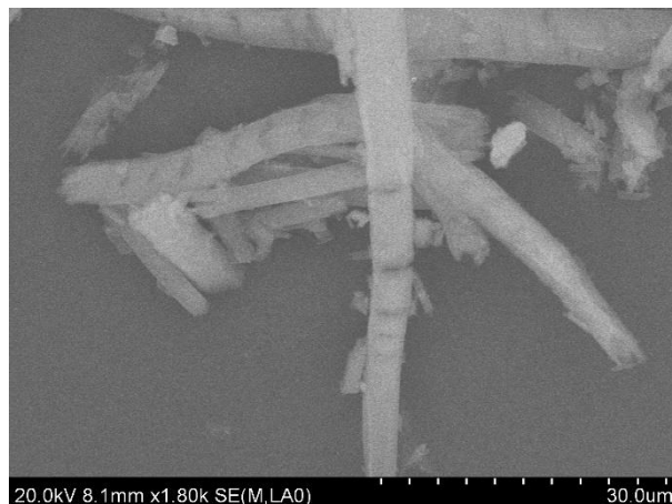
Figure 3.8. SEM image of M2-2 recorded after crystal activation under dynamic vacuum. Scale bars are included in the bottom right corner of the SEM images.
