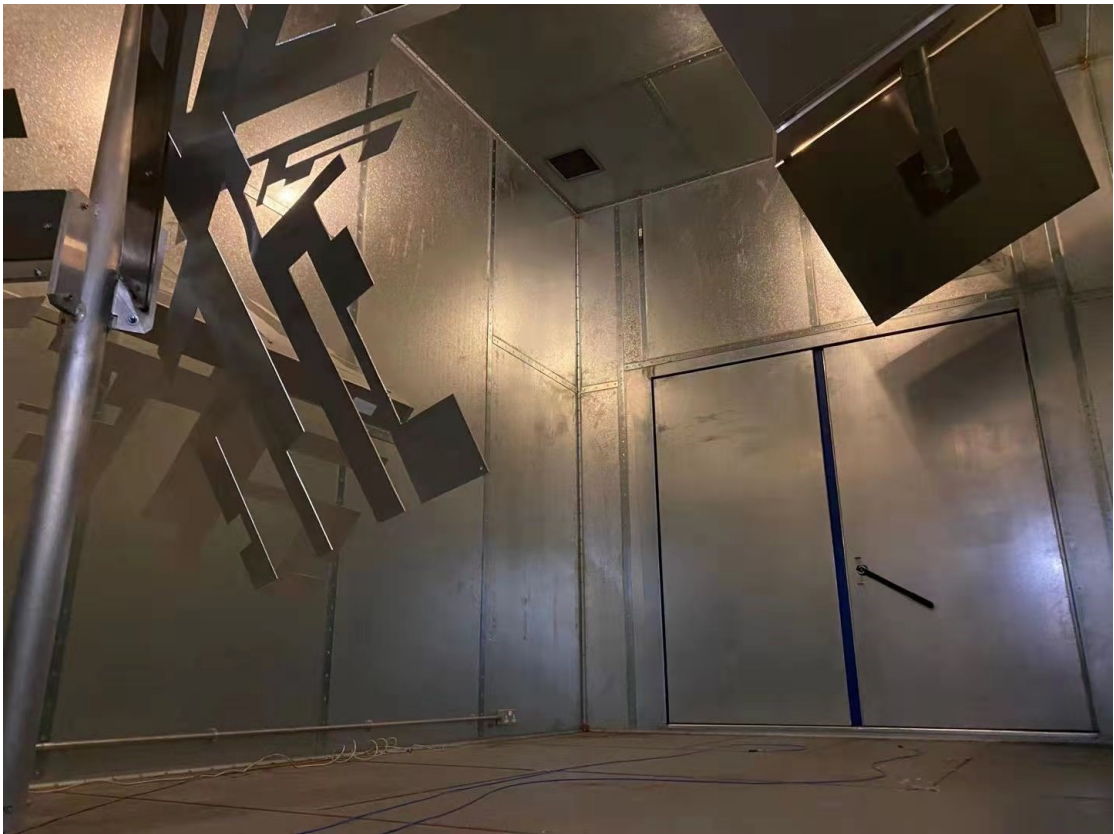
Figure 2.1: A photograph showing the RC at the University of Liverpool with dimensions 3.60 m ( a ) × 5.80 m ( d ) × 4.00 m ( b ).
