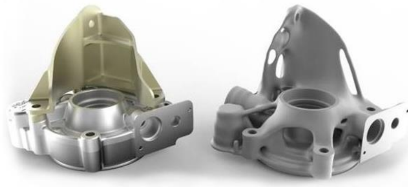
Figure 6: Comparison of front axle differential using traditional manufacturing vs metal 3D printed part [33]
