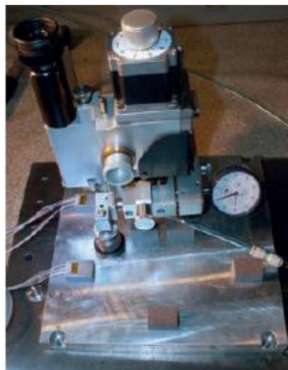
Figure 21: MTS3000 RESTAN (REsidual STress ANalyzer) system by SINT Technology positioned on the construction platform with the samples (from [108]).
