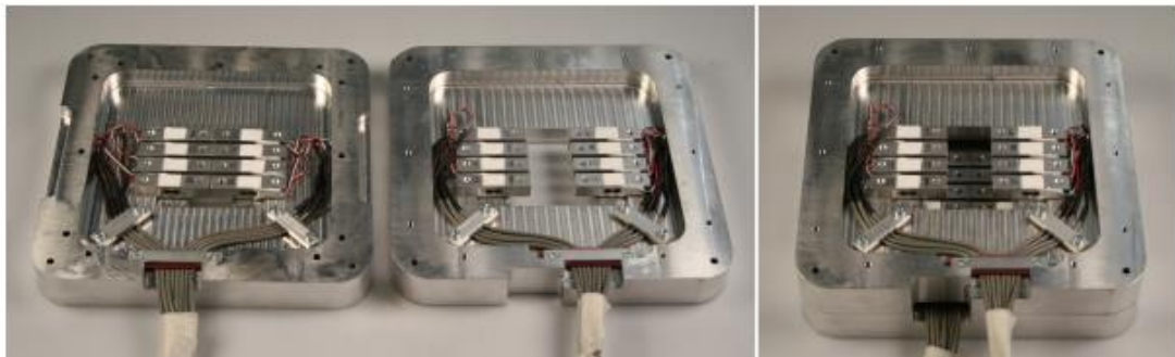
Figure 30: The Force Transducer Device (FTD), developed by Robinson [from 119] for in-situ measurements.
