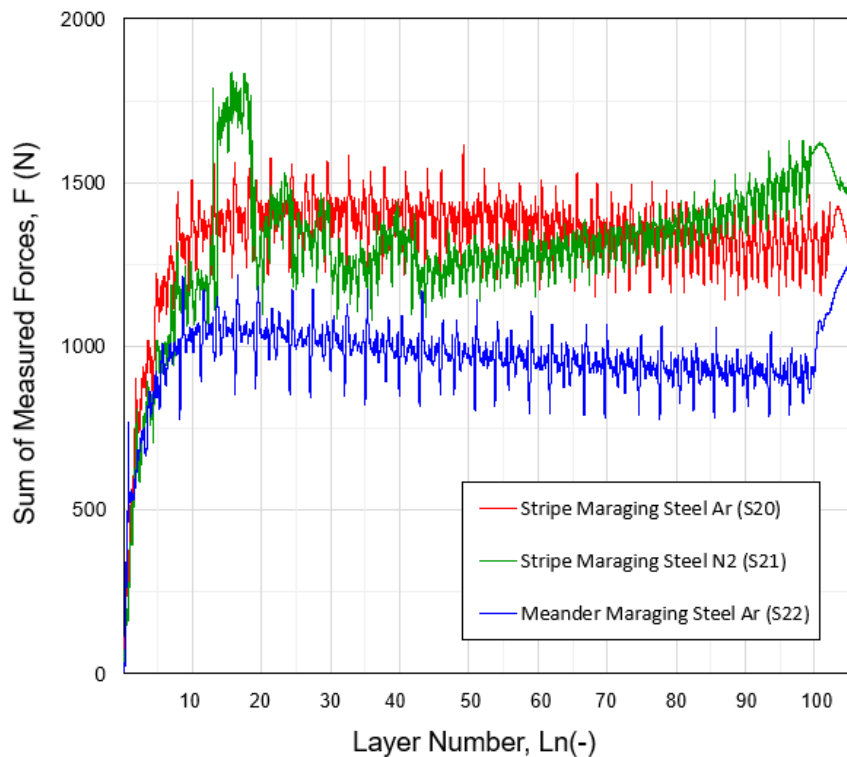
Figure 110: Comparison of the Sum of forces measured in square parts built using Maraging steel using N 2 and Ar as the inert gas atmosphere. Data is shown for parts S20, S21 and S22. For which further details can be found in Table 11.
