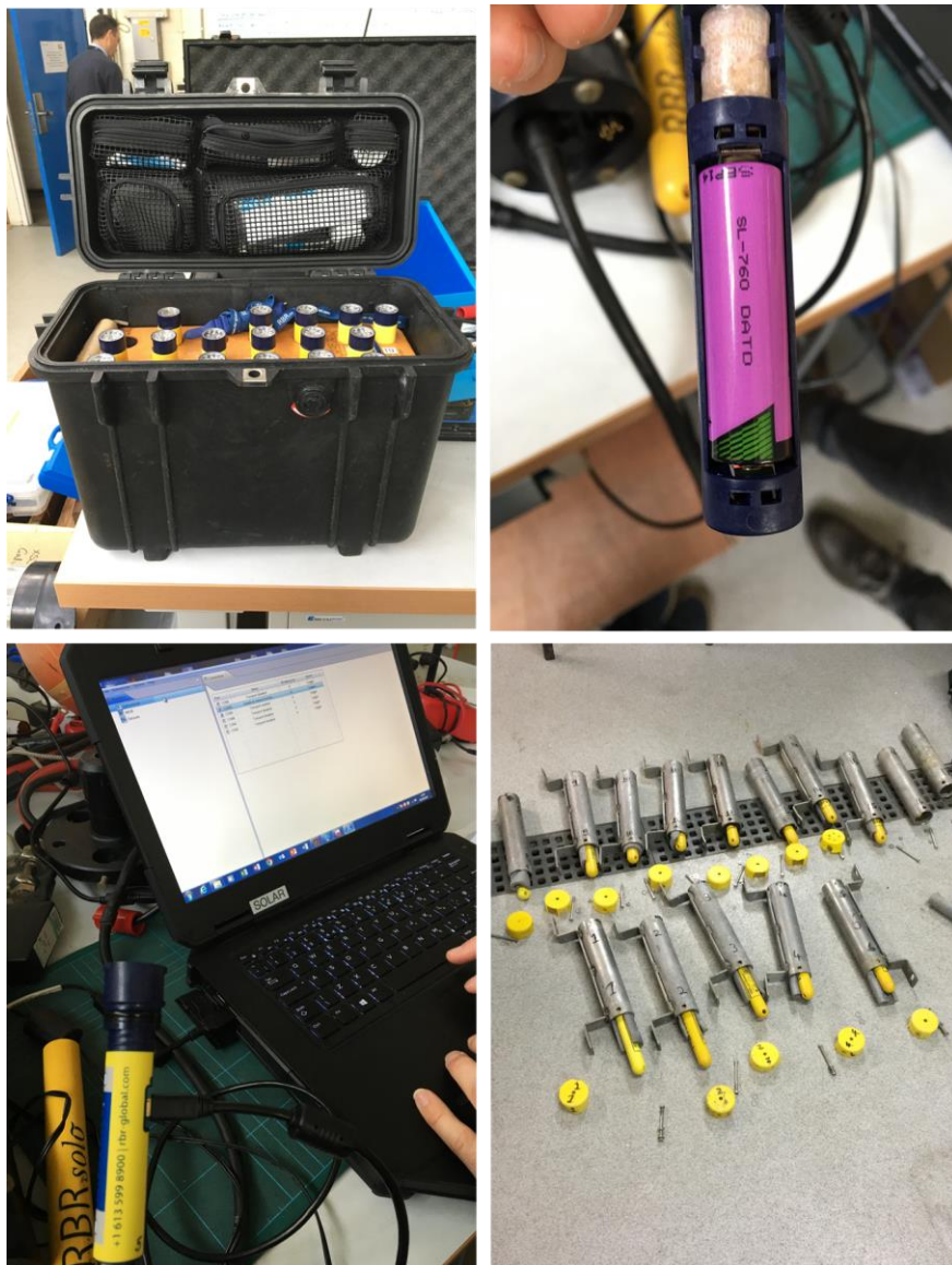
Figure 2-8 Preparing pressure transducers during storm survey mobilization
