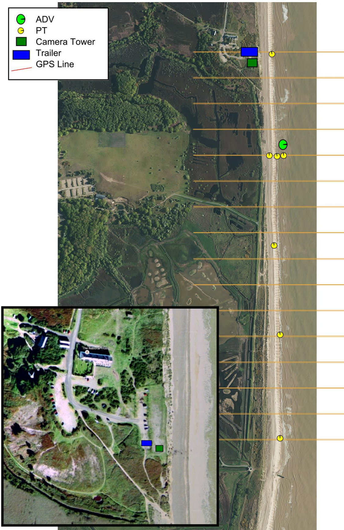
Figure 2, PT locations and Survey lines for Minsmere. 100m profile lines.
