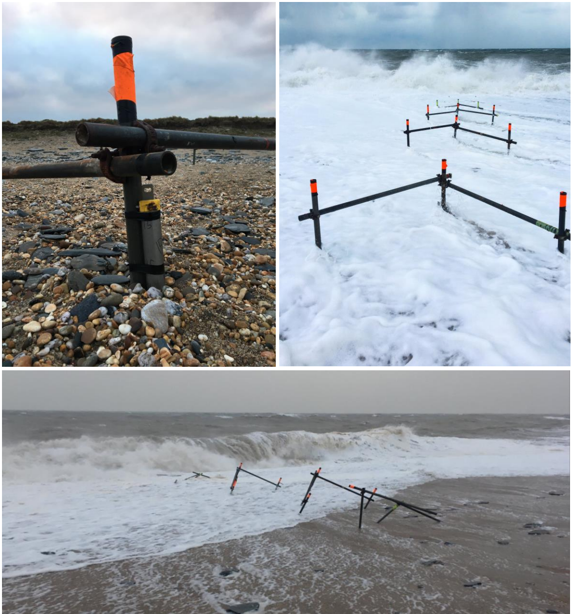
Figure 6-4 Deploying pressure sensor arrays on a gravel beach: Top left: Close up of pressure transducer, in housing, fixed to an arrow head scaffold frame; Top right: Pressure transducer array successfully collecting data through the swash to the inner surf zone during The Beast From The East storm, where offshore wave heights in exceeded of 4 m; Bottom: Damage to pressure transducer array caused by The Beast From the East storm during which offshore wave height exceed 5 m. All photographs taken by the author at Beesands during February/ March 2018.
