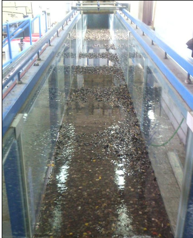
Fig. C. Bed morphology changes after a dam-break flow
