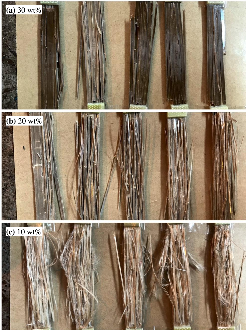
Figure 5.44 Comparison of tensile failure mode for samples with different PAEK–L2O ratio.
