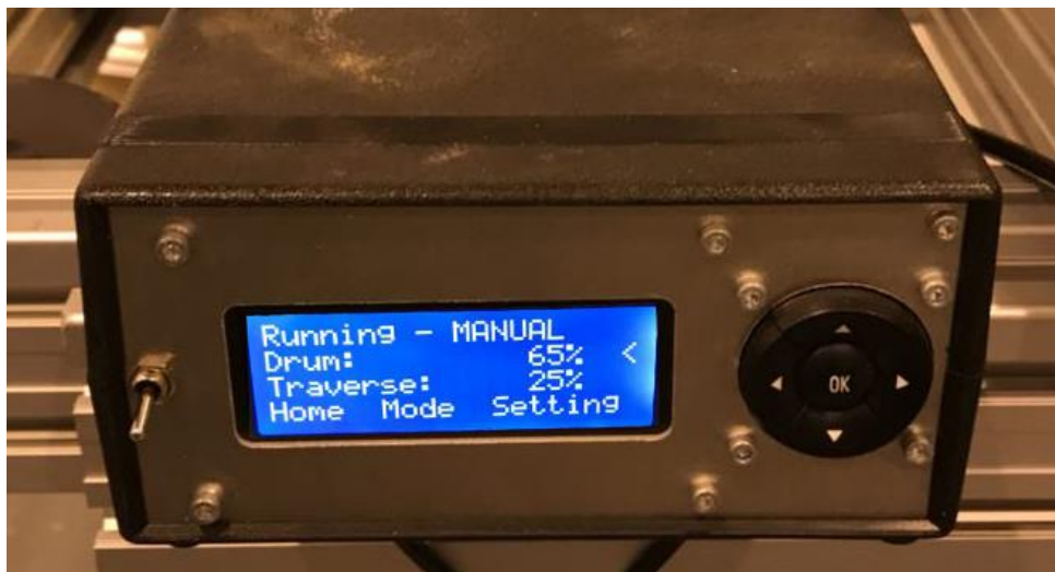
Figure 3.16 Controller for adjusting the speeds of the linear actuator (Traverse) and the winding drum (Drum).
