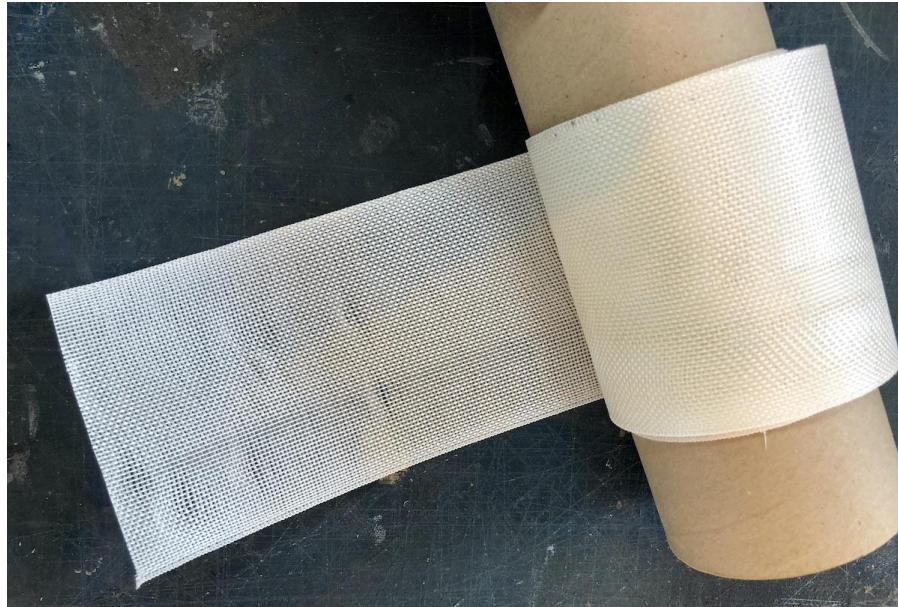
Figure 3.5 Woven glass fibre/PP prepreg manufactured by the trial rig.
