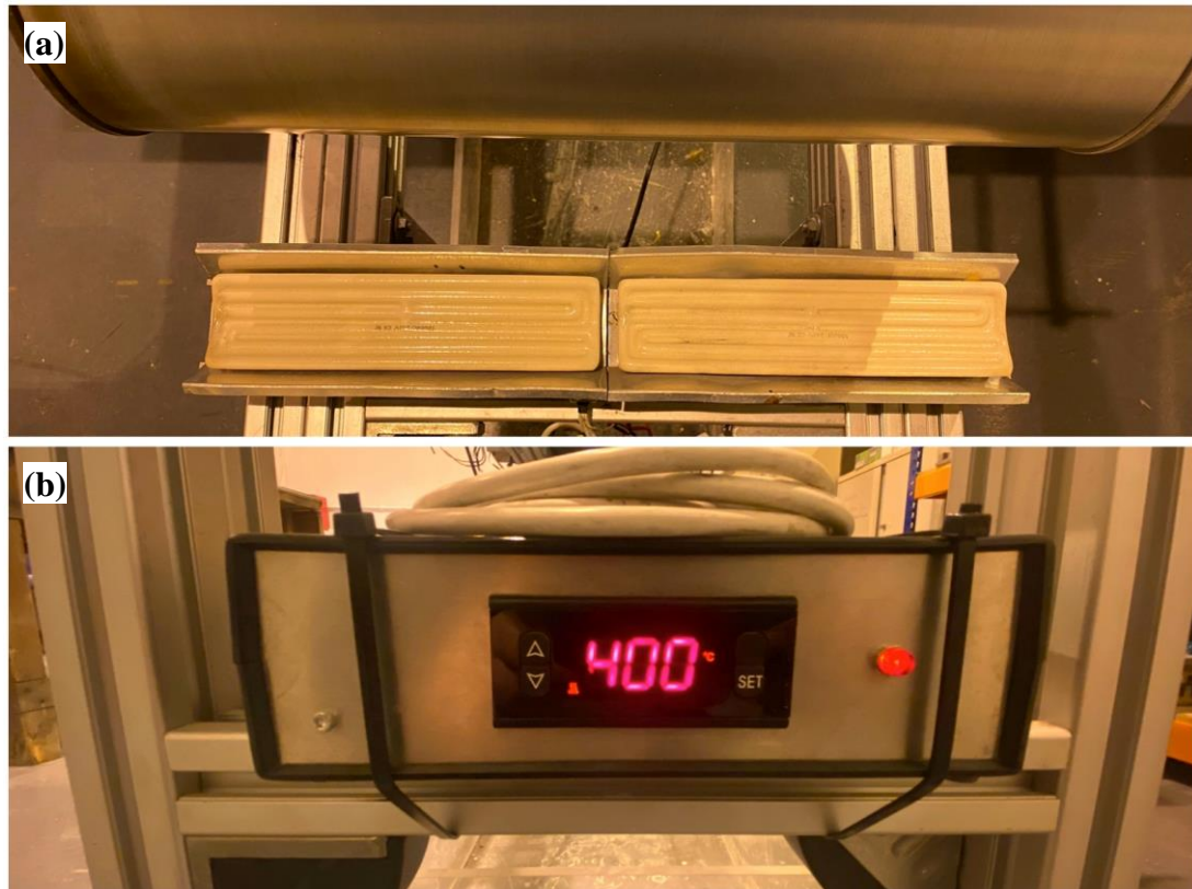
Figure 3.18 The heating unit comprising: (a) two ceramic heaters and (b) temperature controller.
