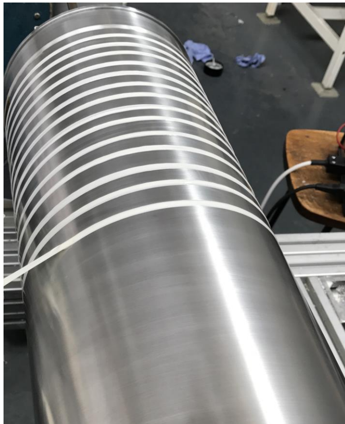
Figure 4.3 Winding impregnated fibre tow on the drum for the resin pick-up test.
