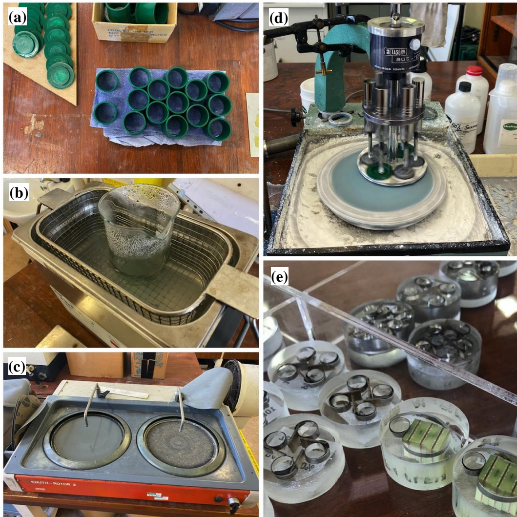
Figure 4.12 The procedure of polishing samples for microimaging: (a) mounting specimens inside 32 mm round moulds, (b) cleaning cured samples in ultrasonic bath, (c) surface grinding, (d) fine polishing and (e) prepared samples.
