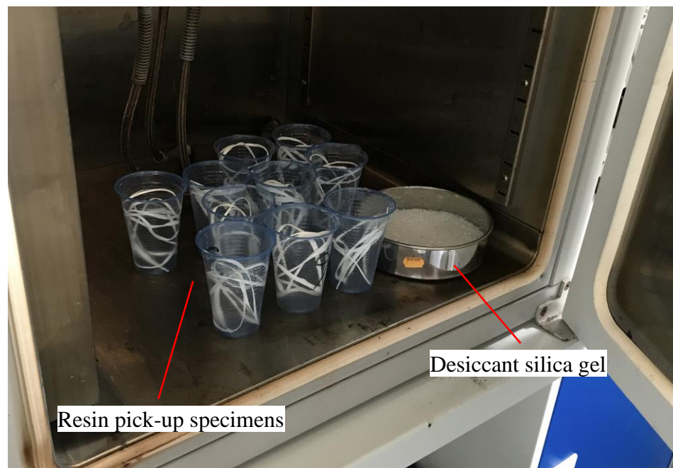
Figure 4.4 Drying process of impregnated fibre tow specimens for resin pick-up test.
