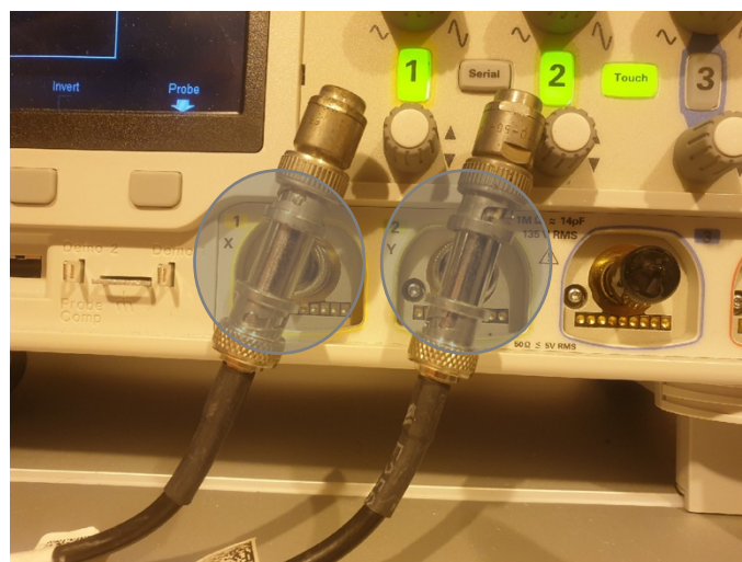
Figure 4.8: Photograph of 50 \Omega resistors (grey shading) used to protect the oscilloscope whilst performing rf -coil cross-talk characterizations.
