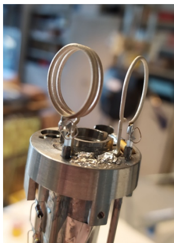
Figure 4.2: Photograph of the perpendicular coupling coils used for inductive detection attached to co-axial transmission cables. The ^1\text{H} channel uses a single loop, whilst the ^{13}\text{C} channel employs three tightly wound loops of smaller diameter. This structure is housed within a brass “cap” whilst in liquid helium. The choice of a cylindrical rf -coil support is necessary to accommodate the sample dissolution stick and to fit into the bore of the polarizer. The two rf -coil loops are elliptical loops of 12 \times 16 mm in diameter.
