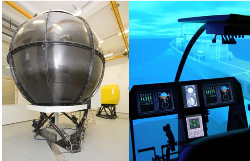
Figure 3 HELIFLIGHT-R simulator – internal and external views
