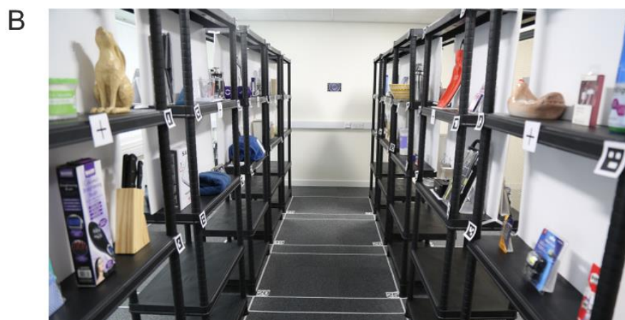
Figure 20. (A) Schematic representation of the mock shop, with 36 shelves across six aisles displaying products. (B) An example of an aisle in the mock shop experiment with floor markers for participant position measurement, fixation crosses for gaze calibration and cardboard stands to ensure front facing view of the product.
