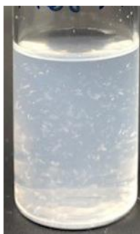
Figure 2.18: Sample stability after 48 hours of dialysis illustrated using the Pluronic® F68: Tween 80 sample.
