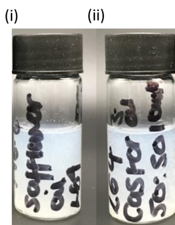
Figure 4.11: Sample destabilisation using Pluronic® L64 as the lone NLC stabiliser for 10 wt% IND dispersions. Representative samples shown were for (i) Safflower oil and (ii) Castor oil.
