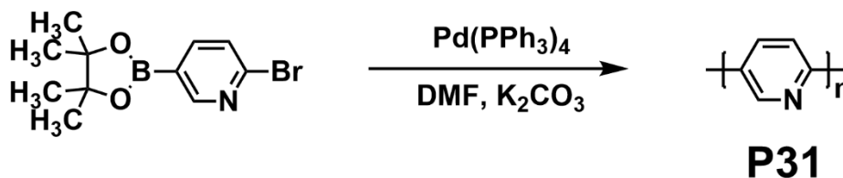
Figure 2.9 Synthesis of P31 via Suzuki-Miyaura-type polycondensation. 16
