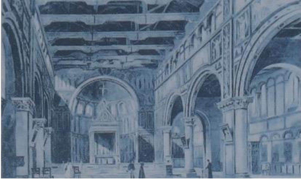
Fig. 28: 1894 interior view by the architect, J. Henry Ball. A different decorative scheme with panels in the arch spandrels is visible with some form of shallow plaster relief over the arches themselves. Sumner followed this lead in his designs.
