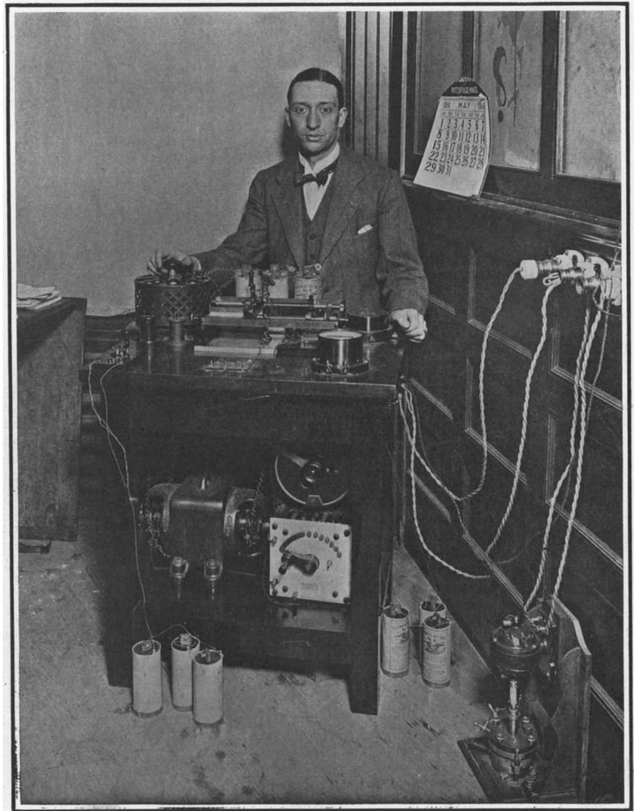
Figure 5. Thorne Baker with his tele-photographic apparatus. Reproduced in Scientific American 102: 21 (21 May, 1910), 417.
