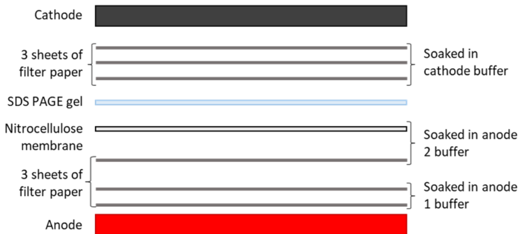
Figure 2.5: Diagram of the semi dry transfer step of a western blot.
