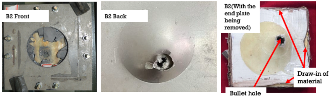
464 Fig. 13. Failure mode of B2 (5 mm SiC + 6 mm compressed wood + 5 mm fabric laminates in total 465 with a 2 mm steel plate): the front face (left), back face (middle) and with back plate being removed 466 (right).
