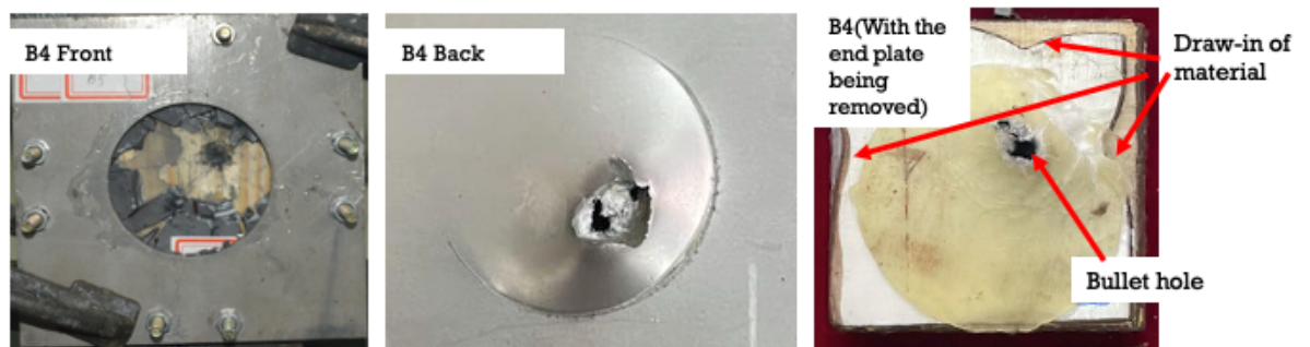
468 Fig. 14. Failure mode of B4 (5 mm B 4 C + 6 mm compressed wood + 5 mm fabric laminates in total 469 with a 2 mm steel plate): the front face (left), back face (middle) and with back plate being removed 470 (right).
