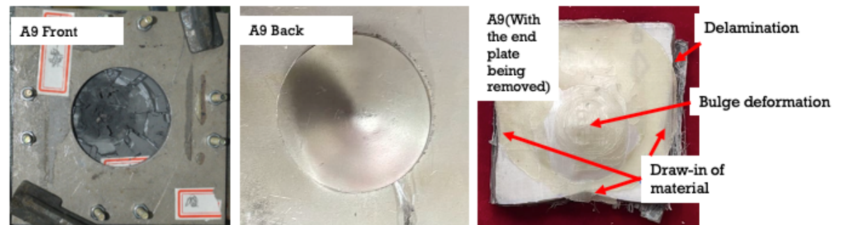
Fig. 12. Failure mode of panel A9 (5 mm B 4 C + 10 mm Dyneema with a 2 mm steel plate): the front face (left), back face (middle) and with back plate being removed (right).
