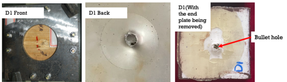
Fig. 16. Failure mode of D1 (15 mm compressed wood + 5 mm Kevlar + 5 mm Dyneema with a 2 mm steel plate): the front face (left), back face (middle) and with back plate being removed (right).
