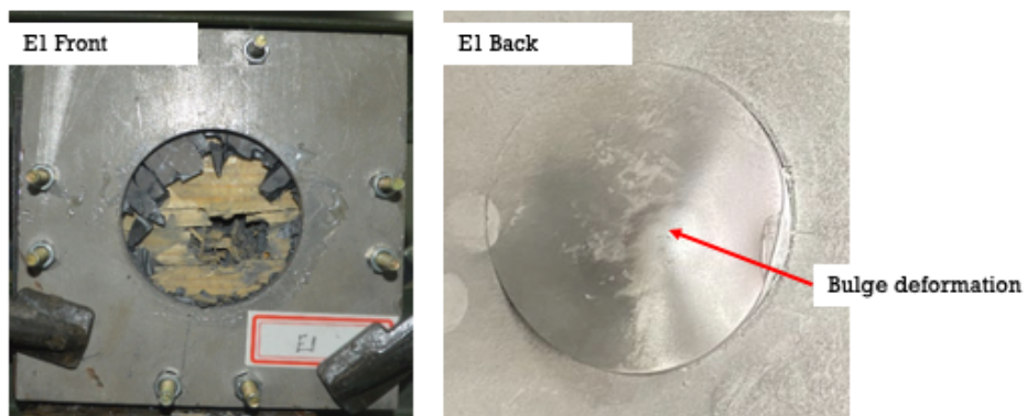
Fig. 17. Failure mode of E1 (5 mm SiC + 4.8 mm compressed wood + 5 mm B 4 C + 2.25 mm Dyneema with a 2 mm steel plate): the front face (left) and back face (right).
