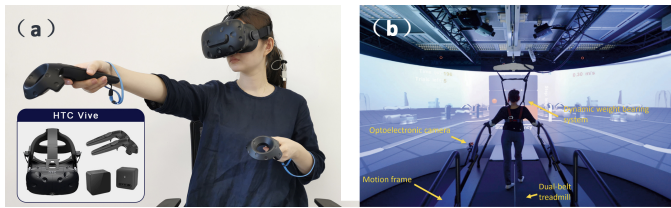
Fig. 2. Built-in motion capture system: HTC Vive (a) and external motion capture system: Vicon (b) [18]
