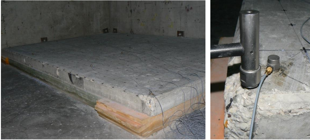
Figure 3-4. EMA measurement set-up using the 21 \times 29 grid for the roving hammer test with positioned accelerometers (left) and an illustrative impact hit on a corner grid point close to an accelerometer (right).
