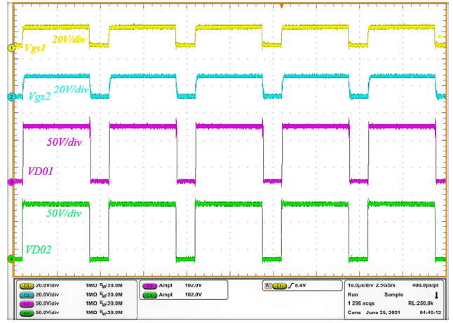
Fig. 18. Gate-source signals ( V_{gs1} , V_{gs2} ) and output diodes voltages ( V_{D1} and V_{D2} ) of the proposed converter. Time ( 10 \mu\text{s}/\text{div} ).
