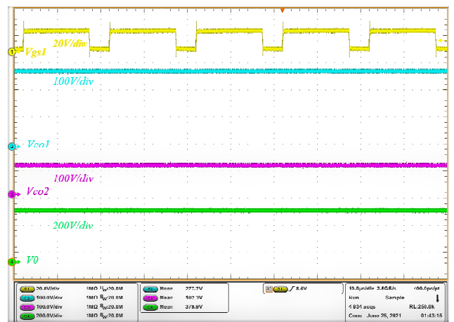
Fig. 20. Gate-source signal V_{gs1} , capacitors voltages ( V_{CO1} and V_{CO2} ) and output voltage V_0 of the proposed converter. Time ( 10 \mu\text{s}/\text{div} ).
