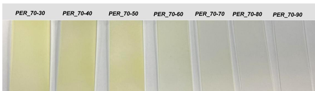
Figure 5.13: Images showing the physical appearance of PER_70-SiO 2 coatings when the weight percentage of SiO 2 was increased from 30 wt % (PER_70-30) to 90 wt % (PER_70-90).
