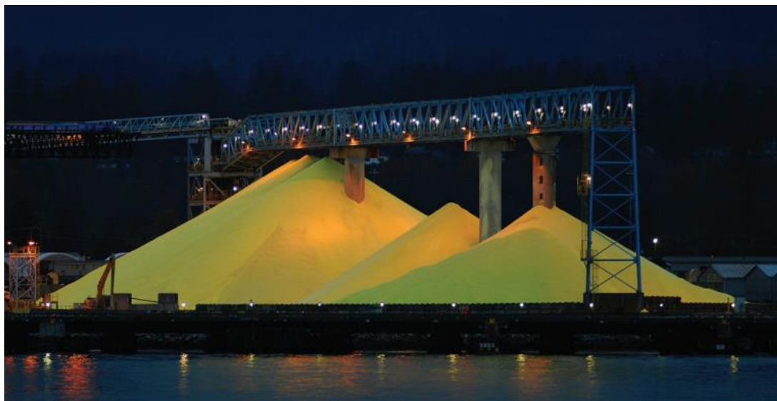
Figure 5.01: A stockpile of elemental sulfur produced from the hydrodesulfurisation process in petroleum refining. Figure taken from ref 10 .
