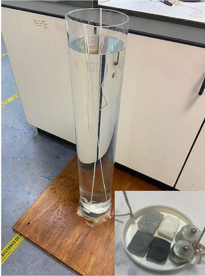
Figure 4.18: Image showing the set-up for periodic submersion measurements of sample set 1, during testing at 7.85 kPa (80 cm depth). Inset; image of the tested samples and sample support/holder.
