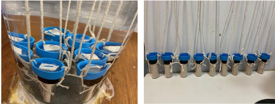
Figure 4.20: Images showing the set-up and individual weighted supports for continuous submersion measurements of sample set 2, during testing at 7.85 kPa (80 cm depth).
