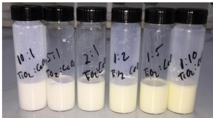
Figure 3.06: Images highlighting the visual pigmentation of blended TiO 2 /CeO 2 -FAS ethanolic suspensions (left to right: 9 wt%, 17 wt%, 33 wt%, 50 wt%, 67 wt%, 83 wt% and 91 wt% CeO 2 ).
