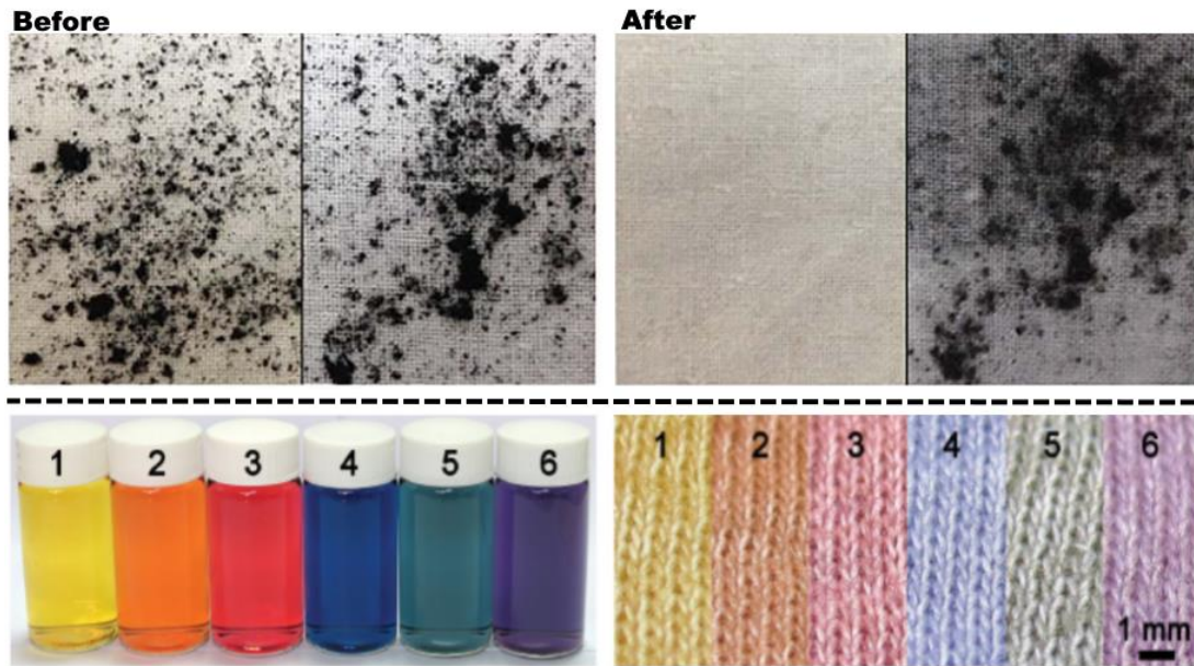
Figure 1.43: Optical images of pristine cotton fabric ( right ) vs treated cotton fabric (coating comprised \text{TiO}_2 nanoparticles functionalised with n-octyl triethoxysilane; left ) with simulated dust particles (pencil shavings), before and after rinsing with water droplets to demonstrate the self-cleaning Lotus Effect on the treated fabric ( top ). Figures taken from ref. 188 Optical images of aqueous solutions of Ag nanoparticles ( left ) and the corresponding dyed cotton fabrics ( right, bottom ). Figures taken from ref. 186
