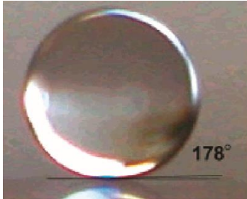
Figure 1.23: Static water droplet with a reported water contact angle of 178^\circ . Figure taken from ref. 70
