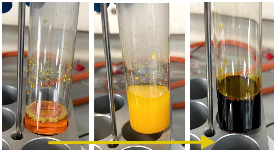
Figure 5.05: Images highlighting the visual changes that occurred when synthesising PER_60, via inverse vulcanisation at >170^{\circ}\text{C} . Initially, the formation of molten sulfur resulted in an orange/yellow solution ( left ), which turned cloudy yellow after the addition of PER crosslinker ( middle ), before finally reaching a deep ruby red, viscous liquid ( right ).
