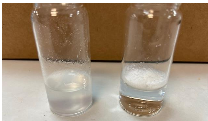
Figure 2.06: Image highlighting the dispersion of as received, unfunctionalised \text{SiO}_2 nanoparticles in aqueous solution ( left ) and HMDS-functionalised \text{SiO}_2 nanoparticles suspending above aqueous solution ( right ), suggesting a change in surface chemistry.
