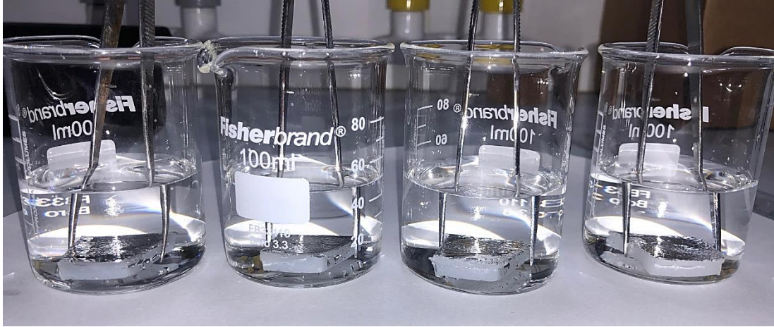
Figure 4.14: Testing set-up – side view of samples submerged in beakers of distilled water at 0.196 kPa (2 cm depth), sealed with parafilm to avoid water evaporation; 0.5-SiO 2 -HDPE (left) ; 0.3-SiO 2 -HDPE (middle left) ; 0.1-SiO 2 -HDPE (middle right) ; and SiO 2 -HDPE (right) .
