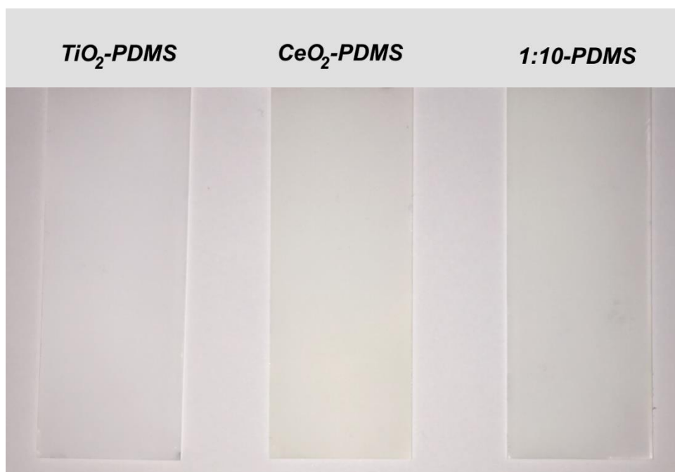
Figure 3.11: Image highlighting the physical appearance of PDMS composite coatings (left to right: \text{TiO}_2 -PDMS, \text{CeO}_2 -PDMS and 1:10-PDMS).
