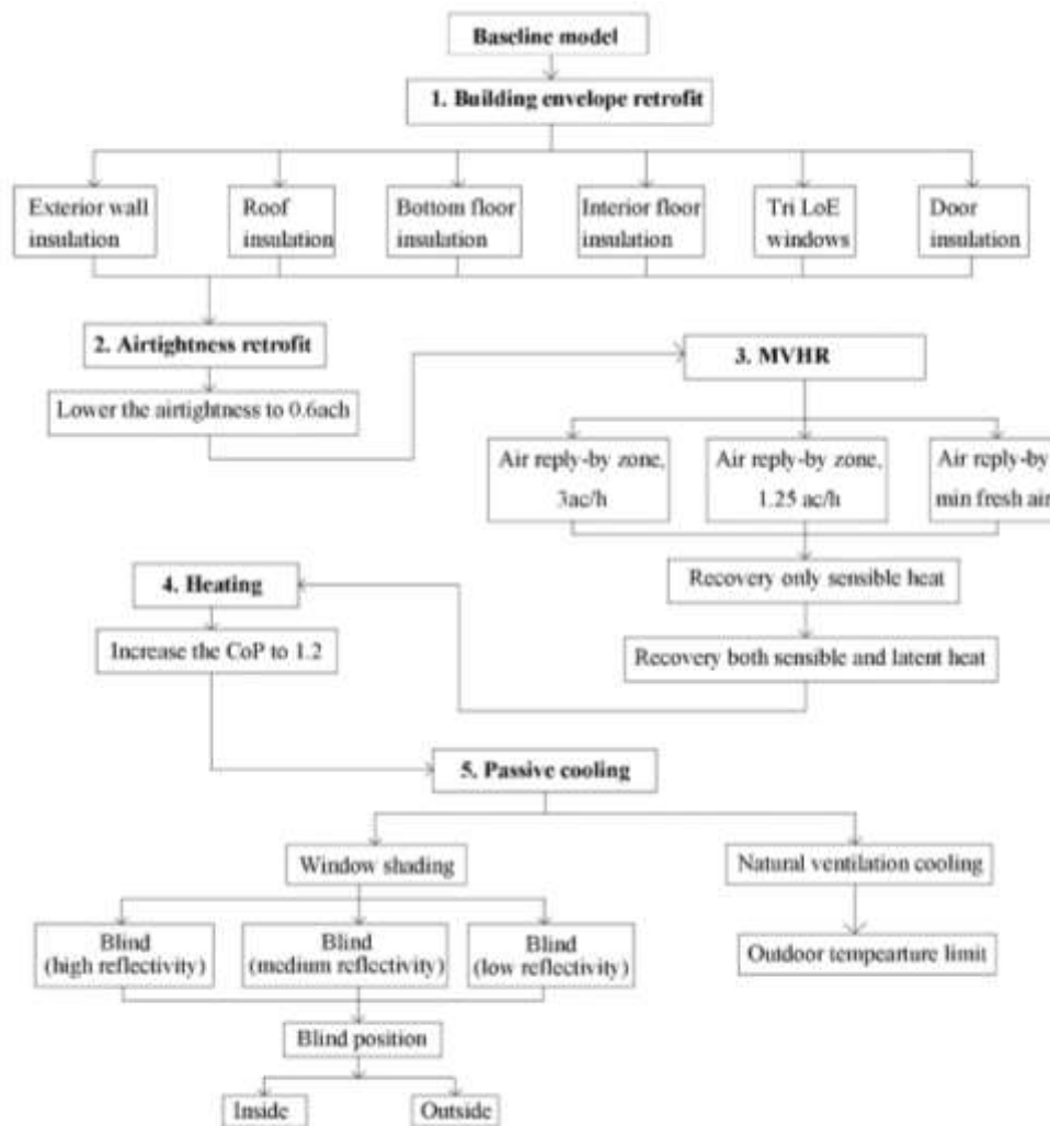
Figure 4-1: Summary of the retrofitting process.
