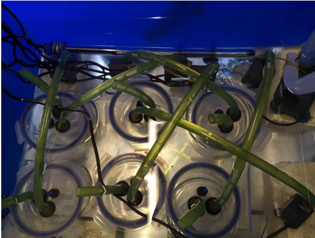
Figure A4.1. Overhead view of apparatus, including 6 intermittent-flow pumps and a chiller pump in the top right corner.
