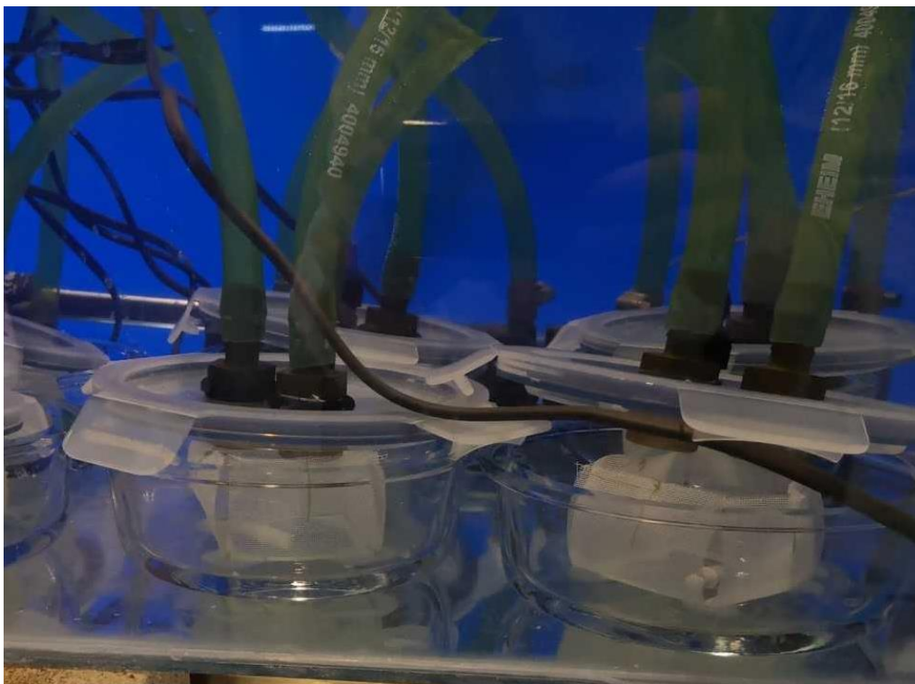
Figure A4.2. Side view of 2 open respirometry chambers, showing external seals and piping.
