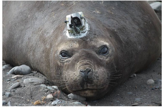
FIGURE 1 Photo of a female southern elephant seal equipped with a CTD Satellite Relay Data Logger
