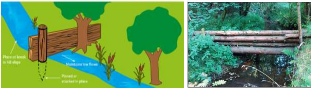
Figure 1. 7 (left) schematic of a Leaky Boards (Woodland Trust, 2016). Figure 1. 8 (right) a woody board installed at Pickering as part of the slow the north Yorkshire flow project (Nisbet et al., 2011).
