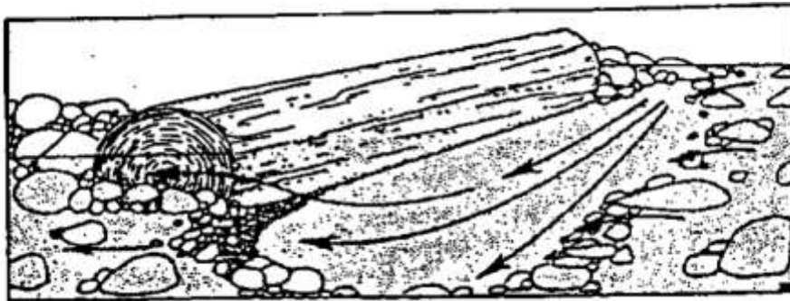
Figure 1. 11 the diversion of flow around a log-jam (Keller and Swanson, 1979)
