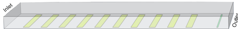
Figure 1.9: The proposed device's schematic, yellow rectangles illustrate electrodes, and green rectangle shows concentration area.
