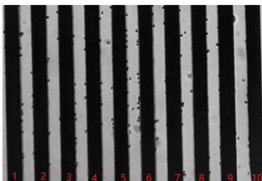
Figure 5.10: Microscopic view of the device (with 50\mu\text{m} interelectrode gap) to show AC pDEP yield for each electrode at 45\mu\text{L}/\text{min} .
