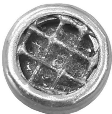
Figure 2. The front of a radium foil cup-style source (R01) showing the dull red-brown foil surface. In this example, the colour is mottled. (The foil is behind the mesh.)
