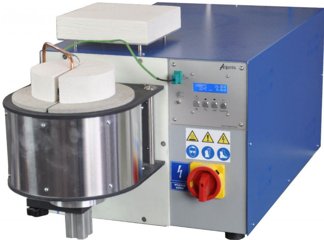
Figure 1.17 - AFI-06 induction furnace purposed for small batch sample making [55]
