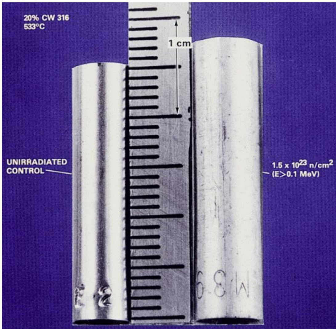
Figure 1.7 - A sample of SS316 showing the difference before and after irradiation to 1.5 \times 10^{23} neutrons \text{cm}^{-2} which has increased its length by 12% [12]
