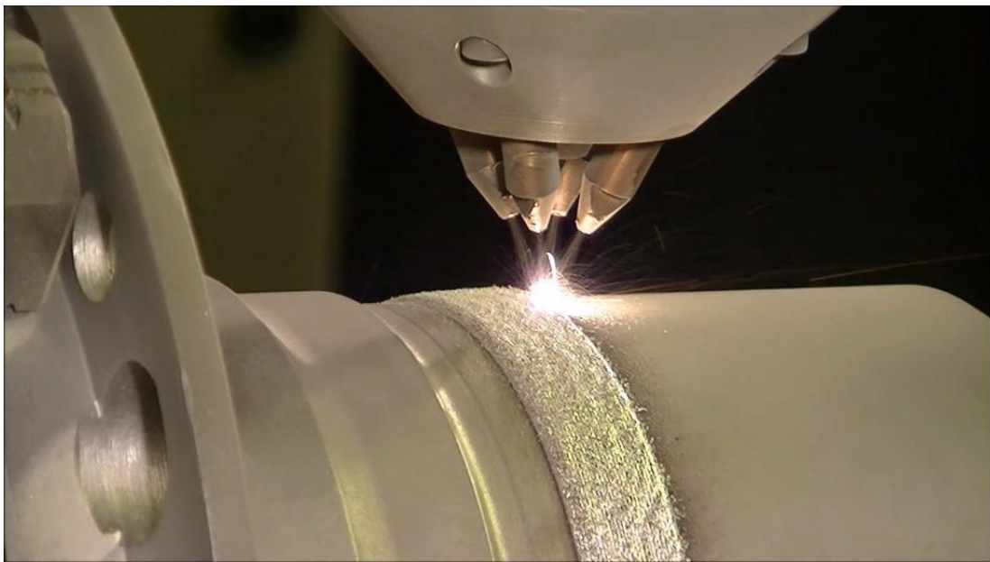
Figure 1.20 - Plasma assist powder 3D print technology, the pre-prepared material powder is spread while the plasma heating the working area [60]
