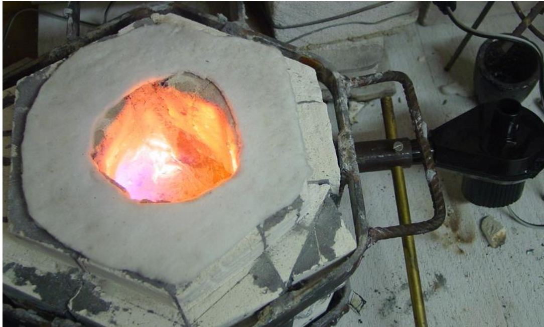
Figure 1.16 - An air burner furnace, with a pool of molten metal.[53]
