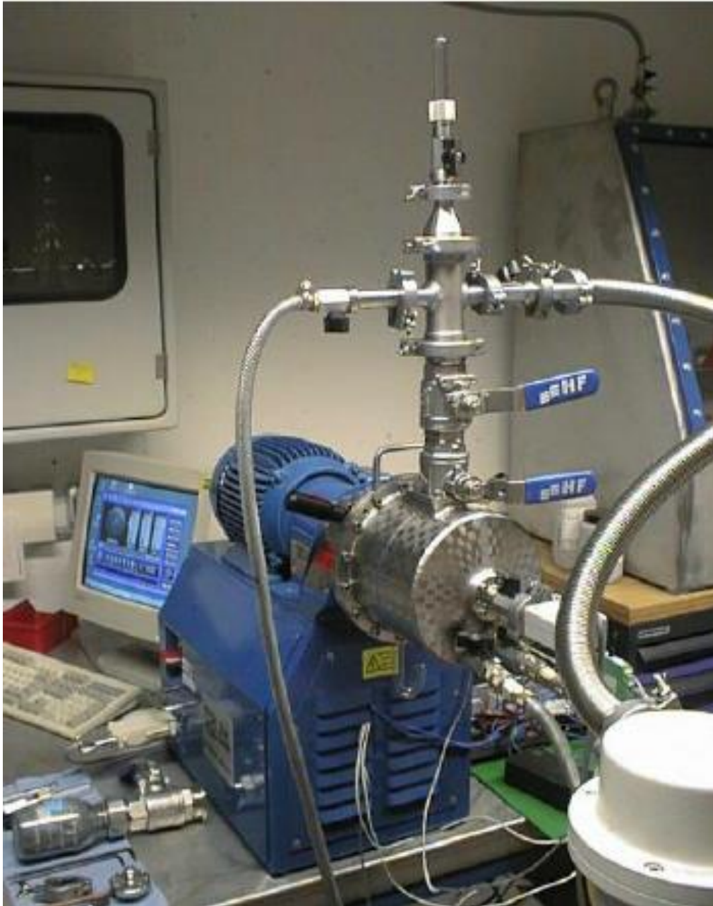
Figure 1.19 - Simoloyer® CM01-2I high energy ball milling with vacuum or inert gas protection [58]
