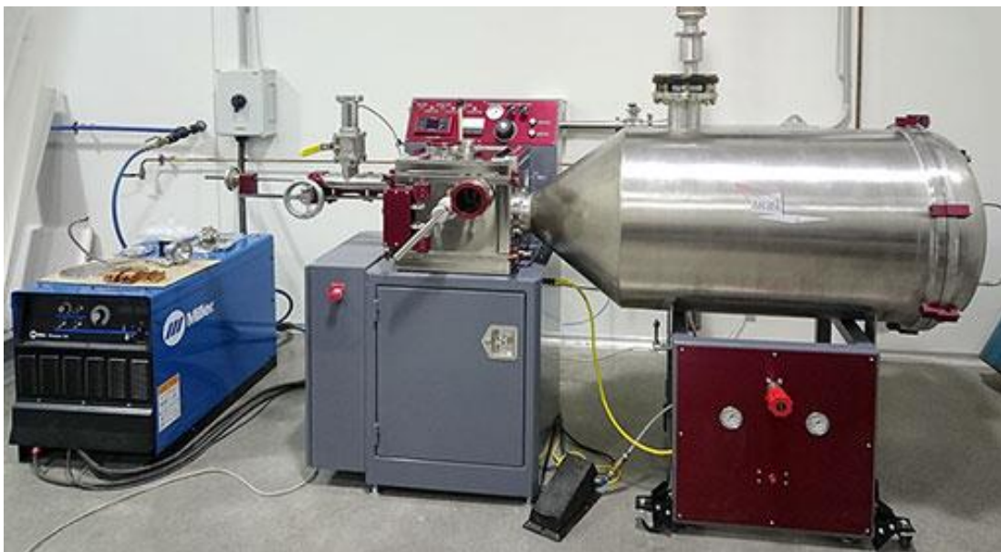
Figure 1.18 - Arc 200 arc furnace which can produce over 3000°C for making high melting point sample [56]
