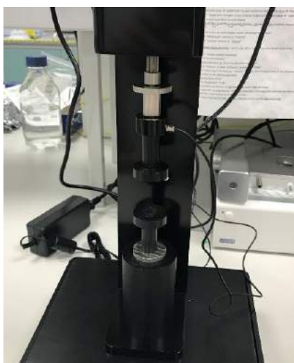
Figure 2.4: CellScale Univert mechanical test system with compression platen set up
