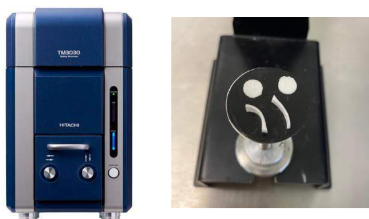
Figure 2.2: Tabletop SEM TM3030 and lyophilized hydrogel top and cross-section visible on SEM stump
