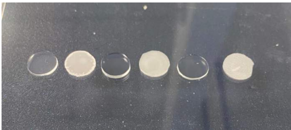
Figure 3.26: Image of macroporous hydrogels from L to R: 30-0.07-Hex, 60-0.07-Hex, 30-0.07-Hept, 60-0.07-Hept, 30-0.07-Oct, 60-0.07-Oct
