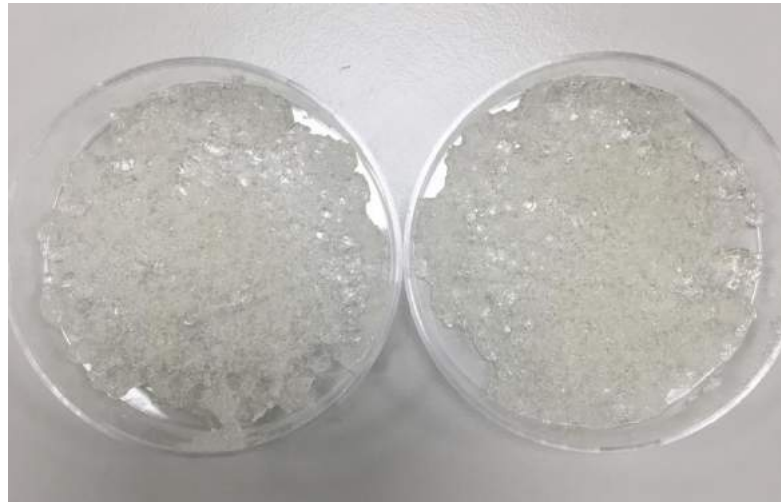
Figure 3.23: Photograph of hydrogel fragments produced when the stirrer device left to run for 1-2 hours. Fragments not stuck together as a sheet and appear opaque. Hydrogel imaged in a 6 cm diameter petri dish. Hydrogel chemistry: 60-0.07-Oct
