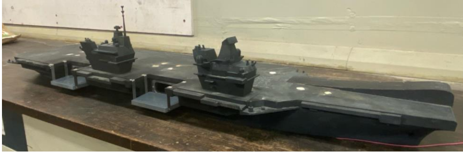
Figure 9. The 3D-printed 1:200 scale experimental model of a twin-island aircraft carrier.
