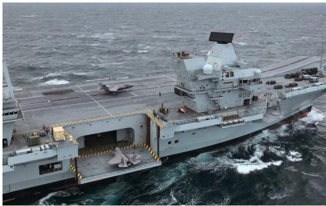
Figure 2. Lowered forward lift of HMS Queen Elizabeth (© Crown copyright Ref. 1).
