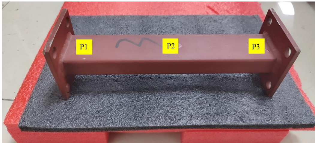
Fig. 4.18 Modal test on the link
