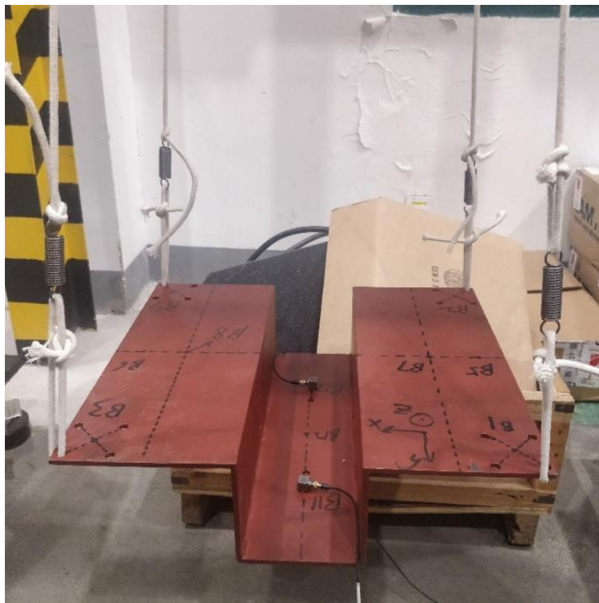
Fig. 4.34 Substructure B under free-free condition
