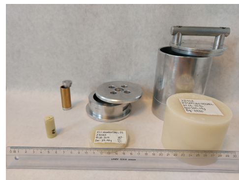
Figure B2. Samples mixed with wax and cast in three different geometries (photo kindly provided by Vicki Hansen, DTU).
