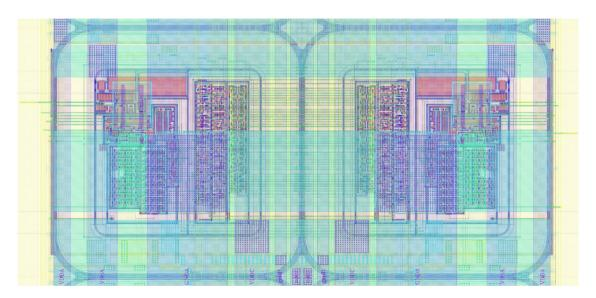
Fig. 5. Layout view of a double pixel. Explanations are given in the text.
