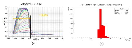
Fig. 2. The simulation of the analogue output gives a ToT of about 30 ns (a) and ToT measurement results show a distribution peaking at 30 ns (b).
