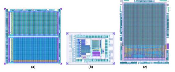
Fig. 1. Layout views of RD50-MPW1 (a), RD50-MPW2 (b) and RD50-MPW3 (c). The dimensions of these prototype sensor chips are 5 mm x 5 mm, 3.2 mm x 2.1 mm and 5.1 mm x 6.6 mm respectively.
