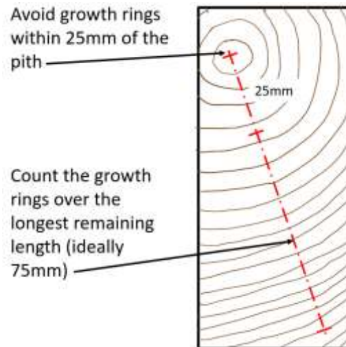
Figure 4.3. The measurement of rate of growth is taken along a radial line, at approximately 90° to the growth rings exposed at each end of a test piece
