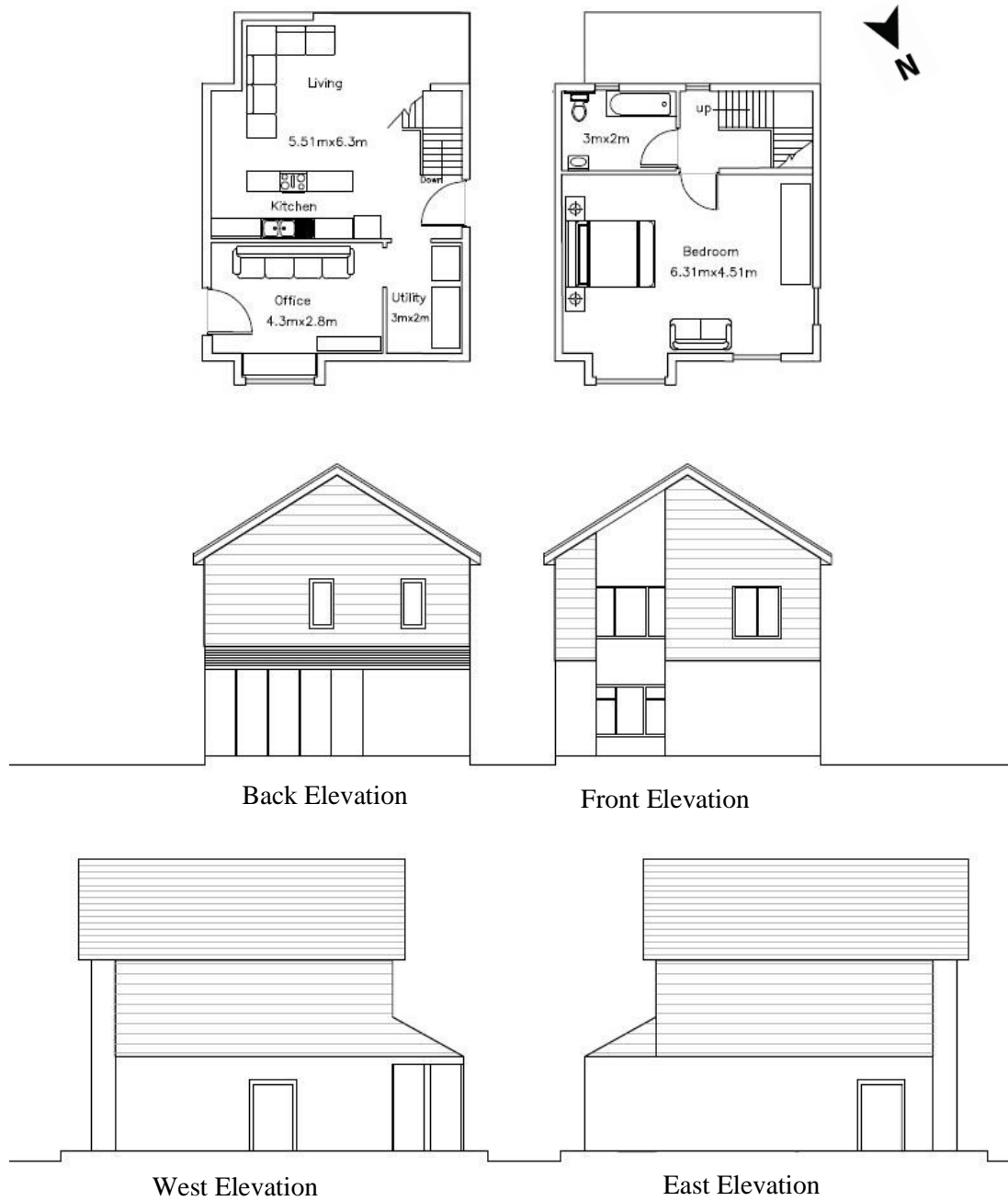
Figure 3. 5: Floor plans, elevations, and section of the SIPs House.(by Author)
