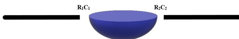
Figure 1.8. Tunnel junctions in series with tunnelling resistances and capacitances, shown as R_1 , R_2 , C_1 and C_2 .
