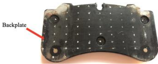
Figure 1.4 Pad model FER7217 with ear and shim removed (Front)
