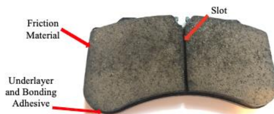
Figure 1.5 Pad model FER7217 with ear and shim removed (Back)
