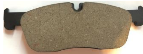
Figure 1.7 Pad model GA8135 without slot (Back)
