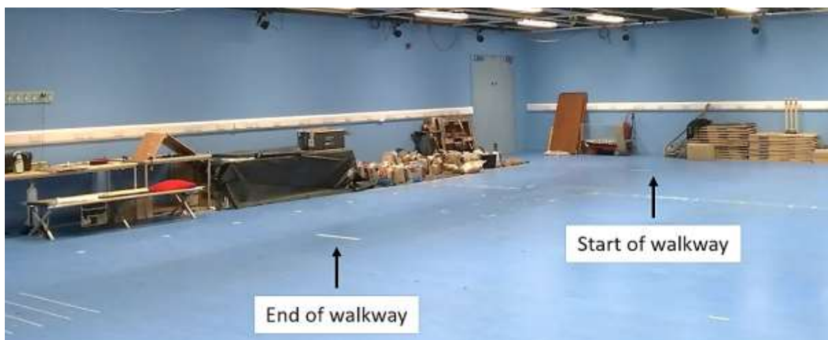
Figure 4. 6. Image of the William Henry Duncan Building gait laboratory with the start and end of the walkway over the force plates (illustrated with black arrows). Each dog was trotted along this walkway containing three Kistler force plates a maximum of 25 times, and for a further 10 walking trials if deemed acceptable and would not hinder the dog's welfare.
