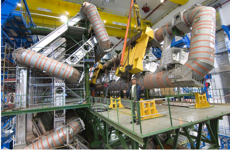
Figure 3.8: A picture showing the real size of the toroidal magnets compared to a person.
