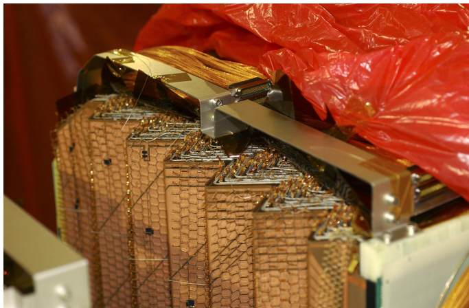
Figure 3.12: A figure of the accordion-shaped electrodes.
