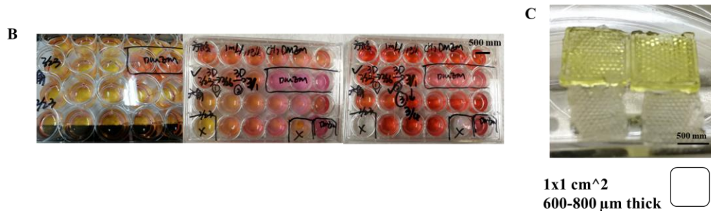
Figure 3.10 Schematic images of the design of leaching test for the 3D-printed PEGDA scaffold A: Four experimental groups designed; B: Images of the preparations for the experimental groups and blank control groups. C: Schematic images of the 3D-printed PEGDA scaffold applied in leaching test.
