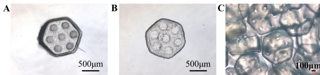
Figure 3.22 The 3D-printed self-assembly PEGDA scaffolds
