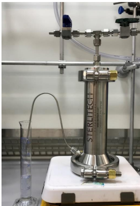
Figure 2.11 To evaluate the separation performance of the CC3-PAN membranes, the permeance and selectivity measurements were carried out using a commercial bench-scale dead-end stirred-cell filtration unit (Sterlitech ® HP4750 stirred cell) that was kept under 10 bar upstream nitrogen pressure at room temperature. The agitation speed was kept at 400 rpm during the measurements. The membrane was cut into a coupon with a diameter of 4.7 cm to fix at the bottom of the cell. Copyright © 2022, Springer Nature and Ai He, etc.
