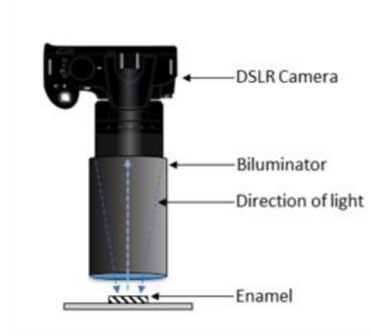
*Figure 2.23: Profile view of QLF image capture set up*
