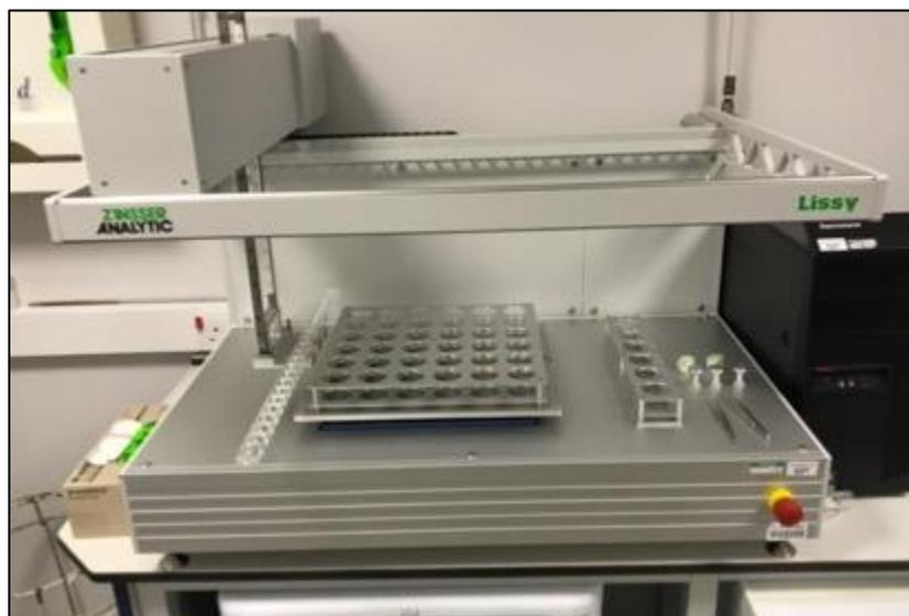
*Figure 2.21 Zinsser Analytic Cycling Robot*
