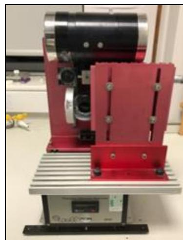
*Figure 2.11 WELL Precision Diamond Wire Saw*
