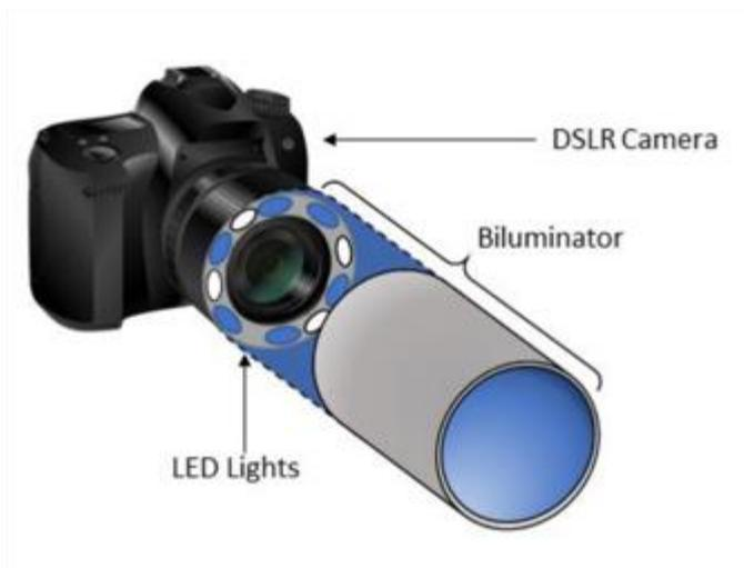
*Figure 2.22: Biluminator and DSLR set up for QLF imaging*
