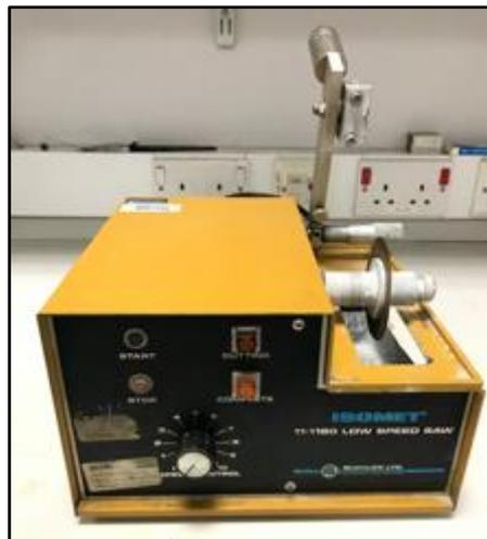
*Figure 2.5 Isomet Low speed cutting saw*
