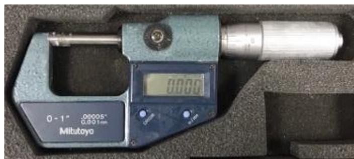
Figure 2.27 Digital Micrometer
