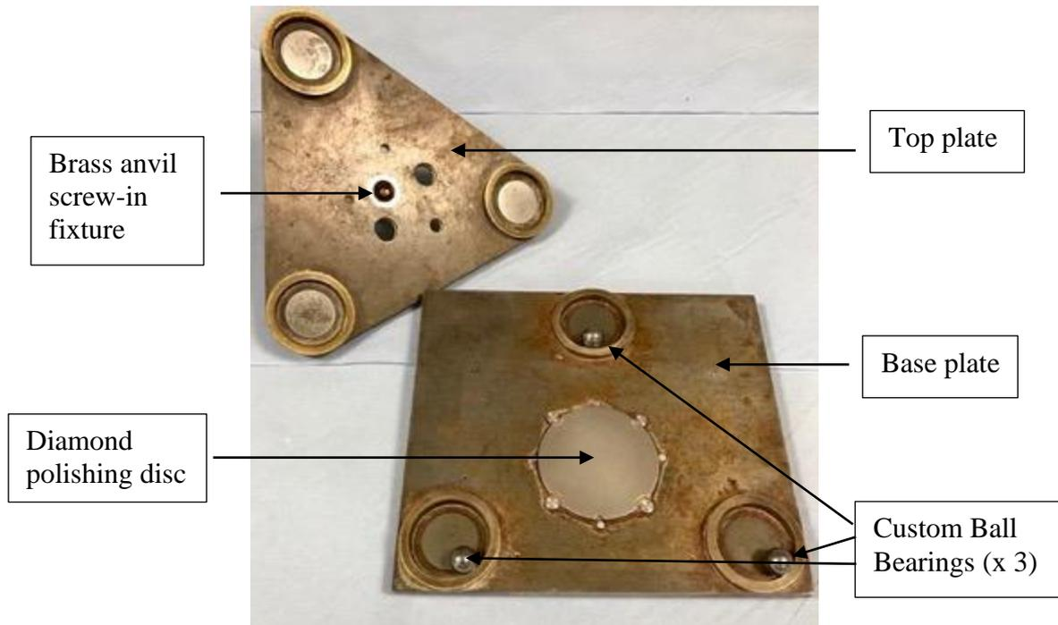
Figure 2.26: Set up apparatus for polishing TMR enamel sections
