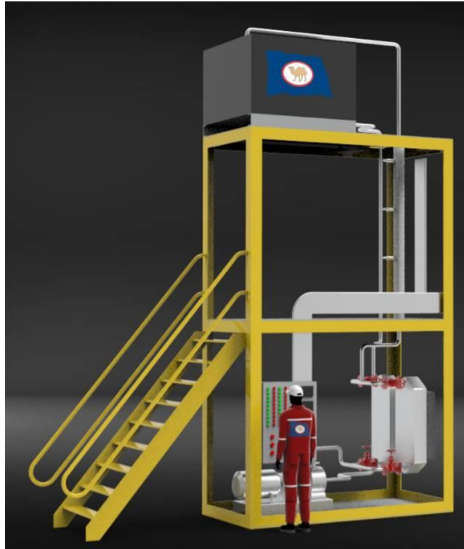
Figure 5-4: 3D sketch of the modular rig with the test section on the right
