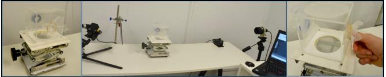
Figure 2.1: Baited box set up. Left: testing chamber placed on an adjustable stand, all sides made with Perspex, with attachable entrance tube, gate and attachable tube for test netting. Middle: whole set up including LED and diffuser, test box and stand and camera lens placed on an adjustable tripod. Right: close up image of the testing chamber with an operator's thumb in position against the test netting.
