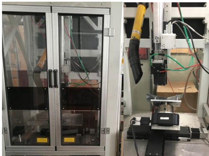
Figure 3.1.6 The CNC moving stage placed in an interlocked cabinet
