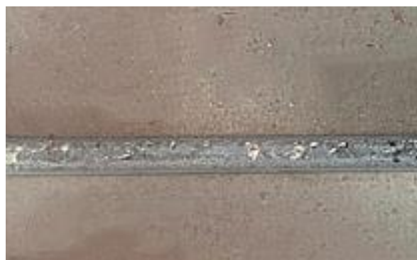
Figure 5.1.2 Mild steel S275, 1.5mm thickness ,5mm Beam Dia., 800W, 30mm/s, surface condition after 20 passes
