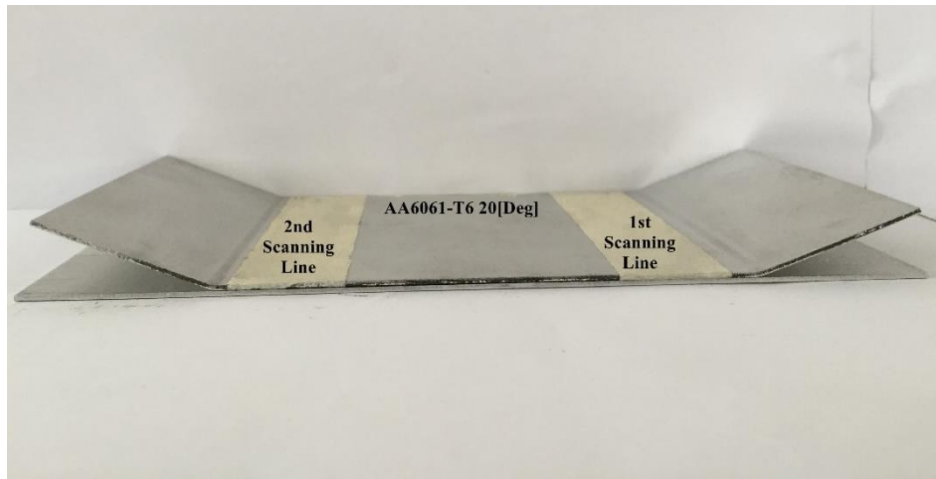
Figure 4.2.13 AA6061-T6 final formed “U” shape component with 20° bending angle
