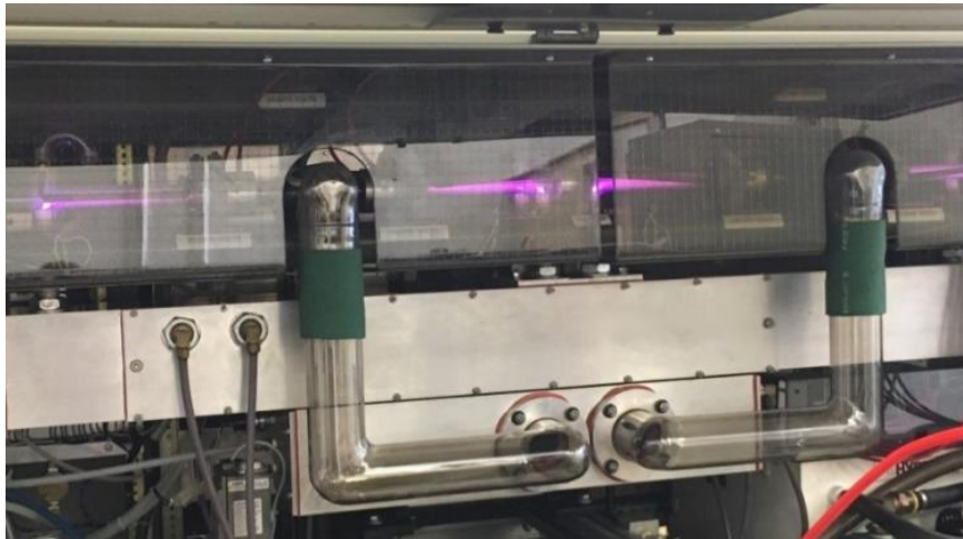
Figure 3.1.2 Laser Cavity, Heat Exchanger and Cavity Discharge
