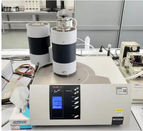
Figure 28. A Netzsch STA 449 F3, a thermal Analysis Instrument.
