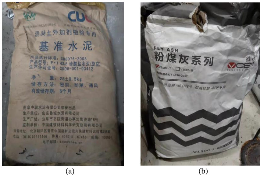
Figure 10 Photos of OPC (a) and FA (b) used in this project.
