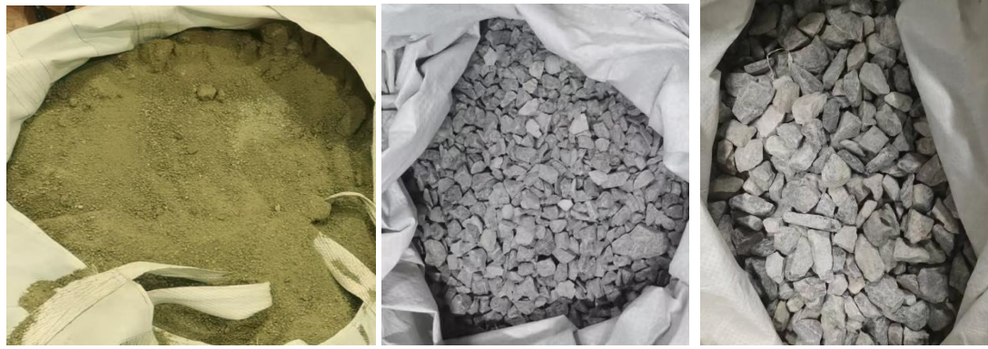
(a) (b) (c) Figure 11 Photo of NFA (a), NCA5 (b) and NCA10 (c) used in this project
