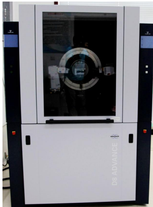
Figure 27. X-ray Diffraction machine, D8 ADVANCE Plus
