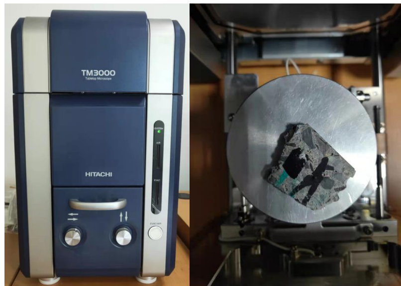
Figure 26. TM3000 desktop electron microscope.
