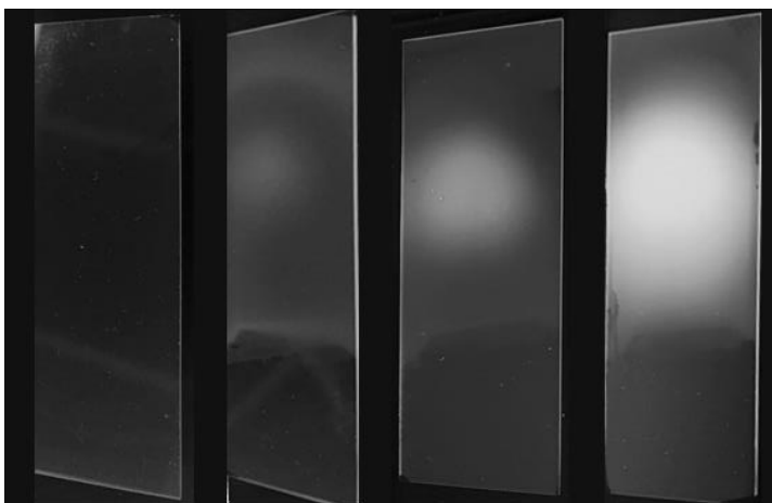
Figure 2.9: PDMS coating on glass substrates deposited using ta-AACVD at activation temperatures of (from left to right) 200, 280, 360 and 400°C. Note; the glass slide shown are microscope slides of typical dimensions (75 x 25 mm).
