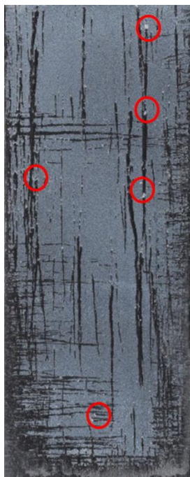
Figure 3.11: Scanned image of PDMS coating after 10 abrasion cycles. The image shows that for some parts of the coating, although has been removed leaving a scratch behind, they curled and remained hanging on the surface instead of being completely detached. This can be seen as brighter white dots on the image, like those highlighted with red circles.
