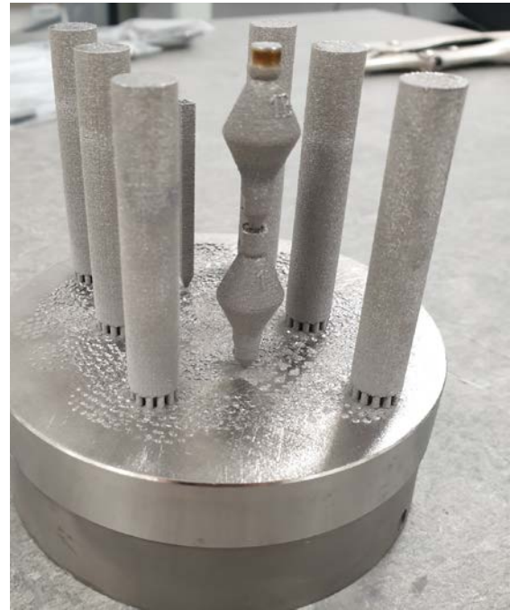
Figure 91: Image of build layout and control tensile build from the TRUMPF TruPrint 1000.
