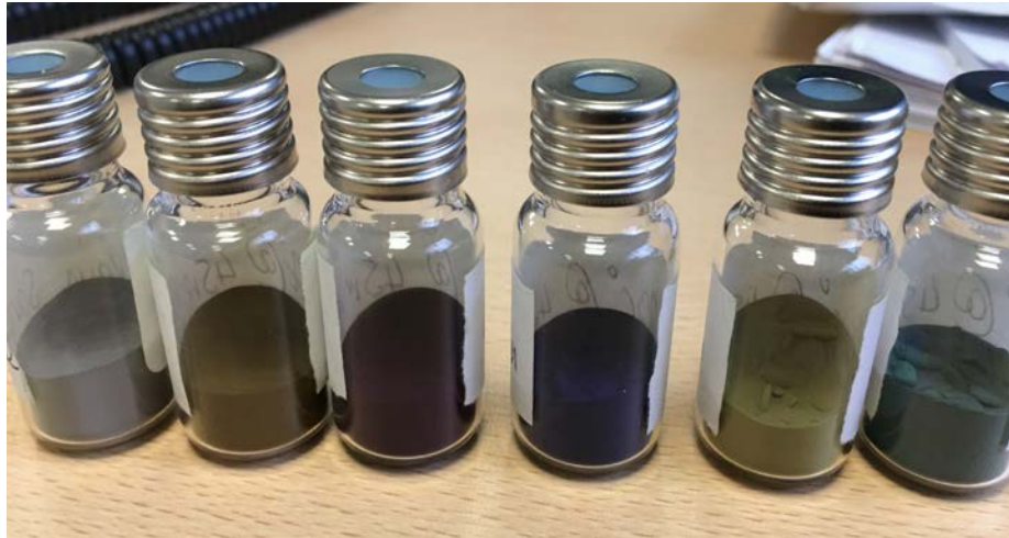
Figure 47: Thermally oxidised Ti-6Al-4V powder particles; ranging from virgin (far left) to green (far right).
