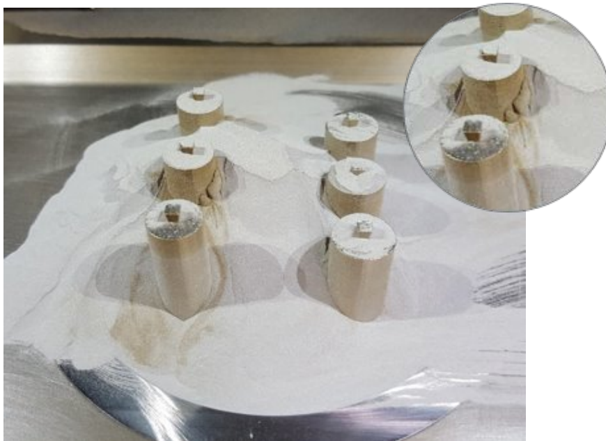
Figure 85: Image of heat affected zone powder surrounding Ti-6Al-4V parts inside the TRUMPF TruPrint 1000.
