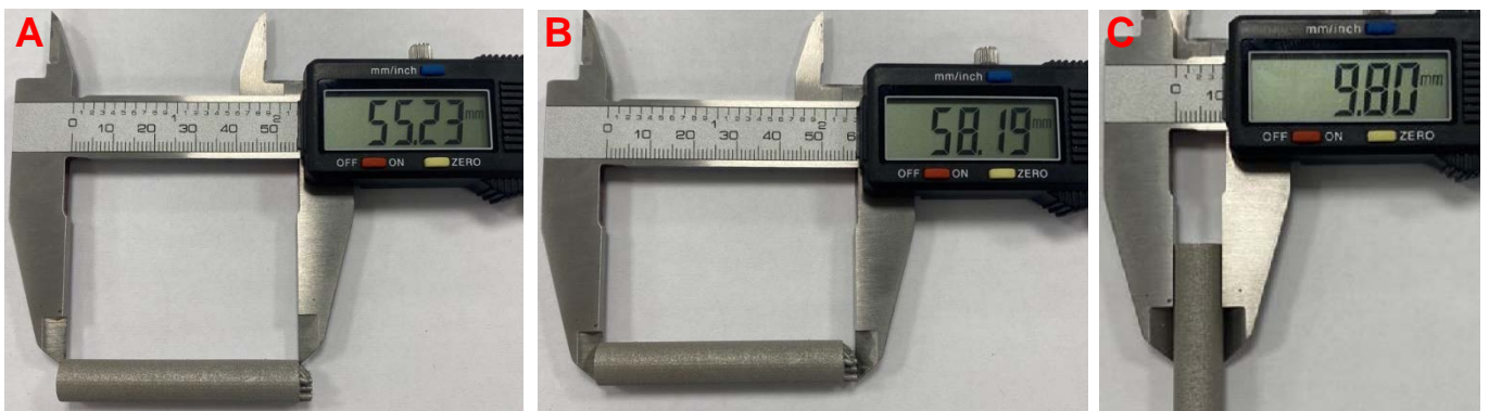
Figure 92: Dimensions of as built tensile bar: A) Length of bar excluding support, B) length of bar including support and C) diameter of bar
